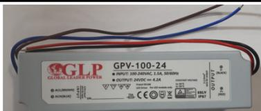
GPV-100-24 Toiteplokk LED valgustitele 100W DC 24V/4A sisend 100-240VAC, IP67, L190xW53xH37mm, hall
